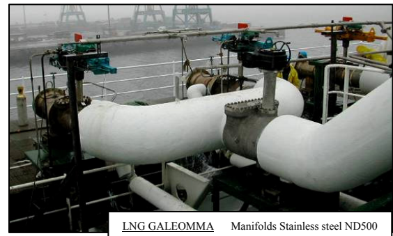
LNG GALEOMMA Manifolds Stainless steel ND500
